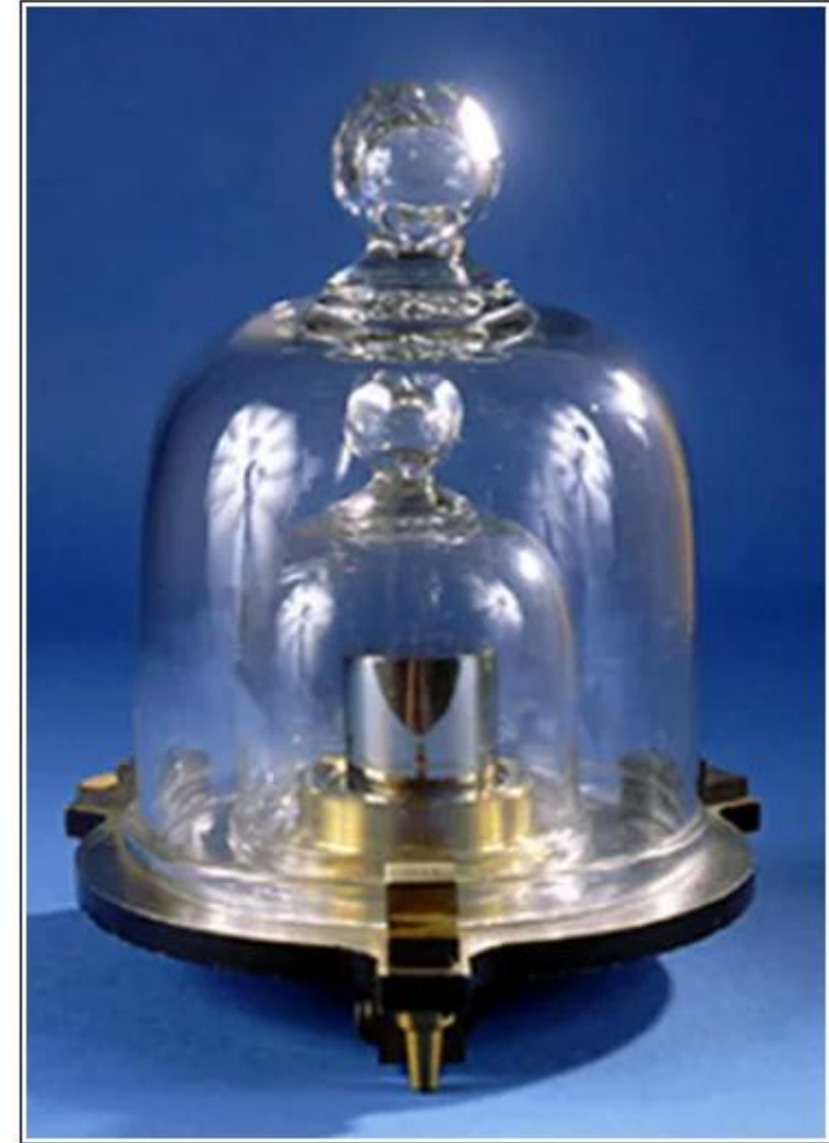
Figure 1.24 This replica prototype kilogram as previously defined is housed at the National Institute of Standards and Technology (NIST) in Maryland. (credit: National Institutes of Standards and Technology)
